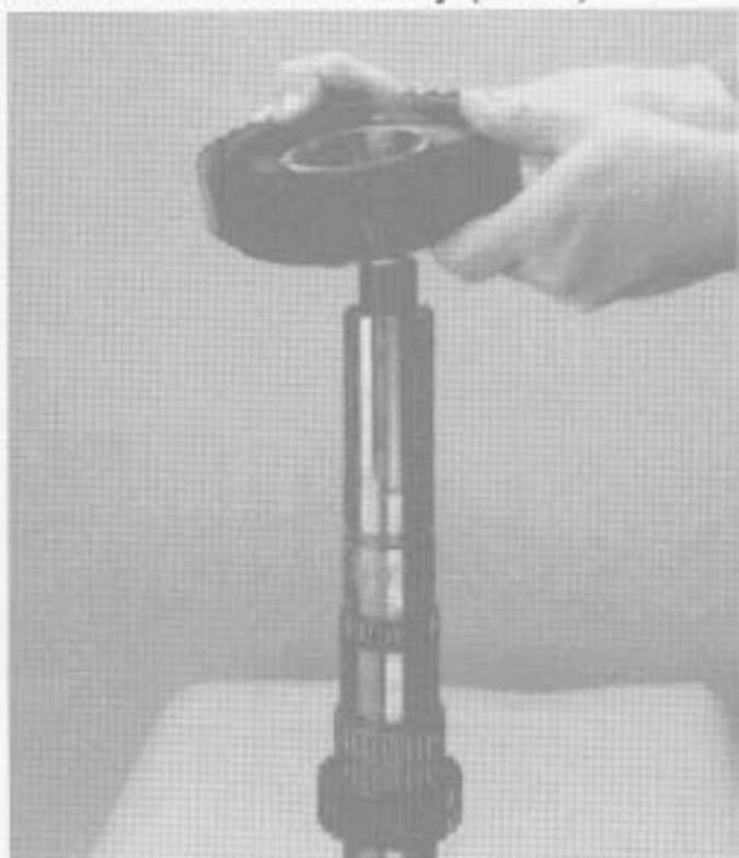
27. Remove 2nd speed gear.
