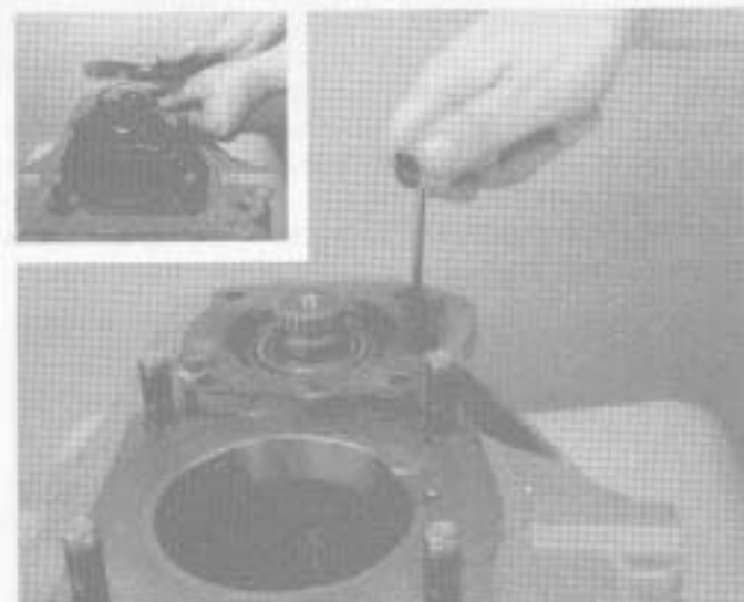
12. Temporarily install new shims into the bearing retainer (inset). Install the retainer and tighten the set screws to the recommended torque.
