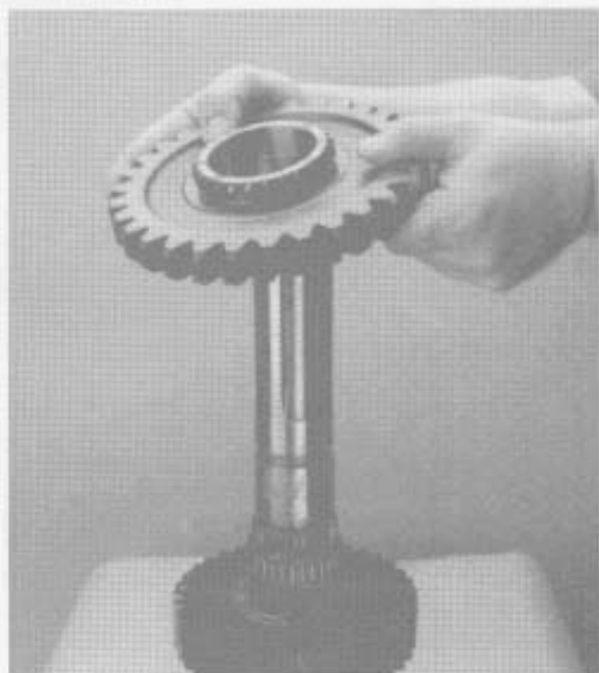
6. Install mainshaft reverse gear.
