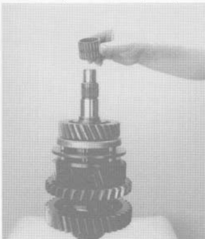
21. Install mainshaft 4th gear bearing.
