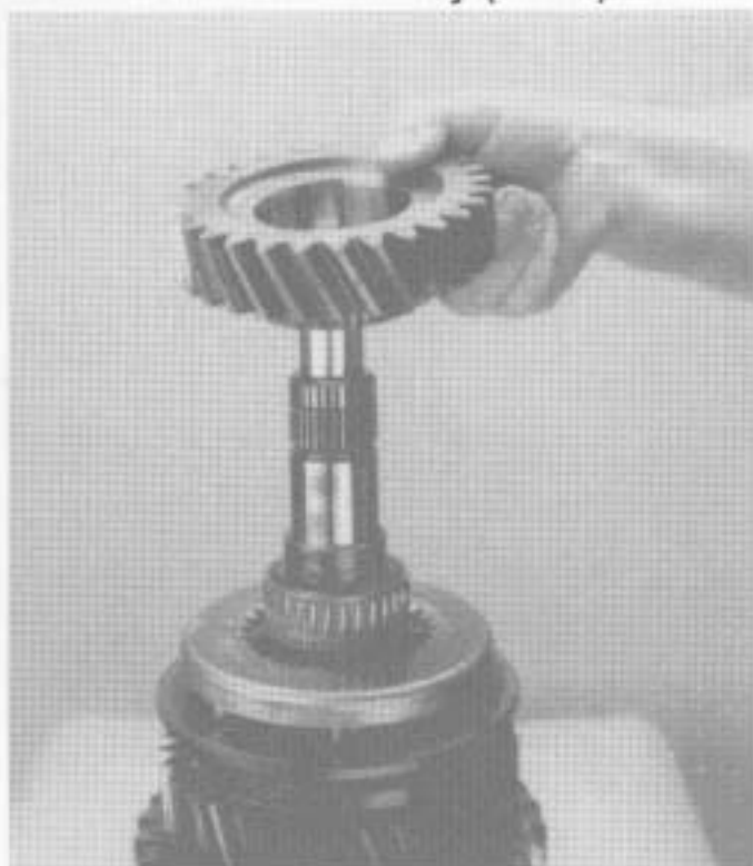
11. Remove the 3rd speed gear.
