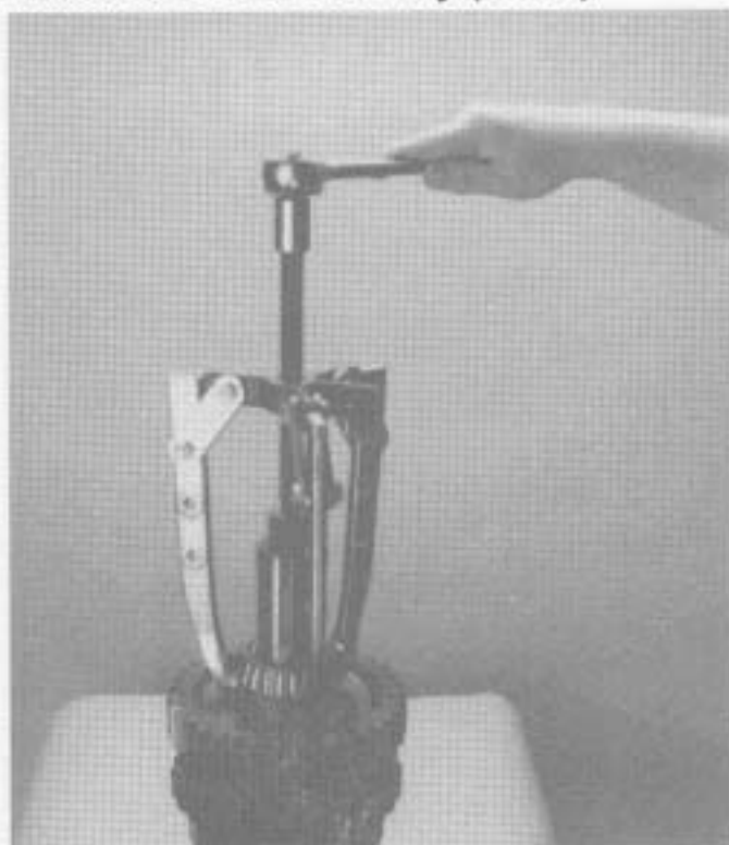
15. Using a gear puller, remove the mainshaft rear bearing as shown.
