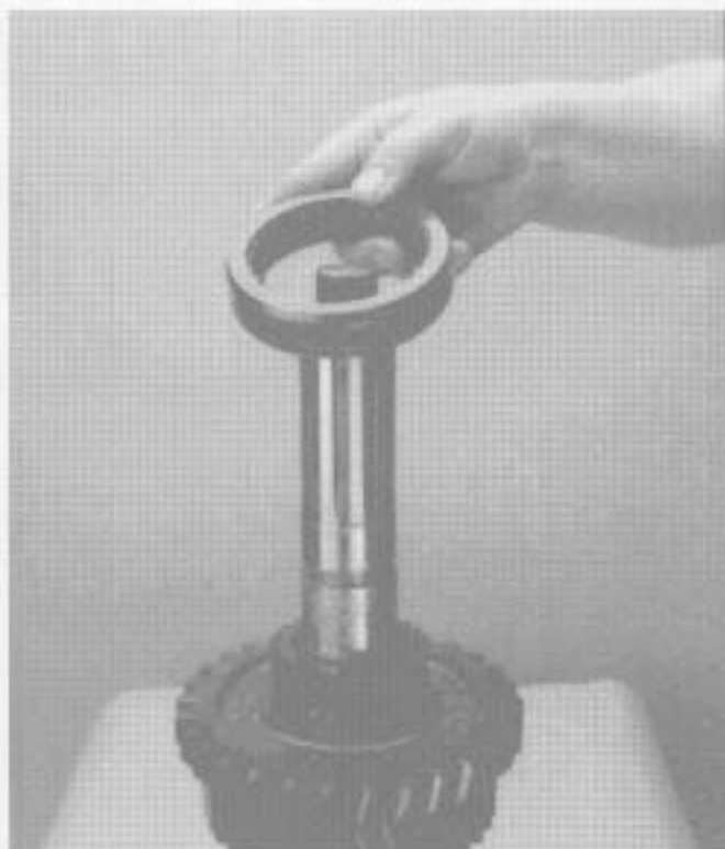
21. Remove the 1st-reverse sliding clutch.
