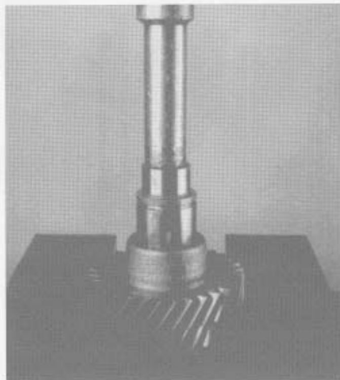
12. Remove countershaft 4th gear.
