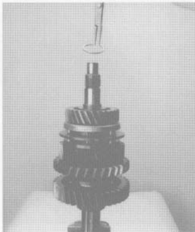
9. Remove 3rd speed gear retaining snap ring.
