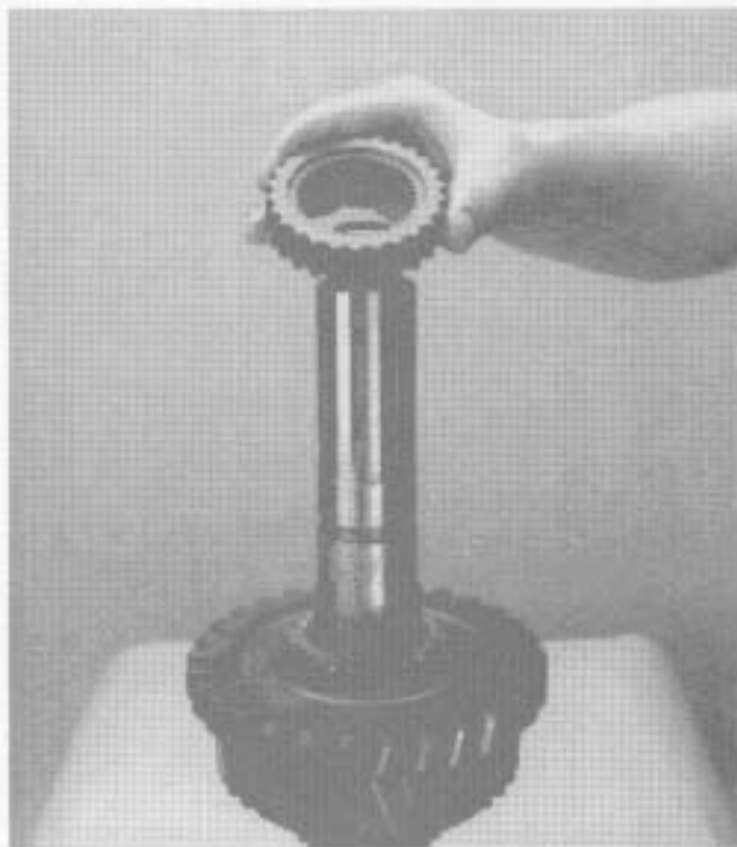
7. Install mainshaft 1st-reverse speed clutch hub.
