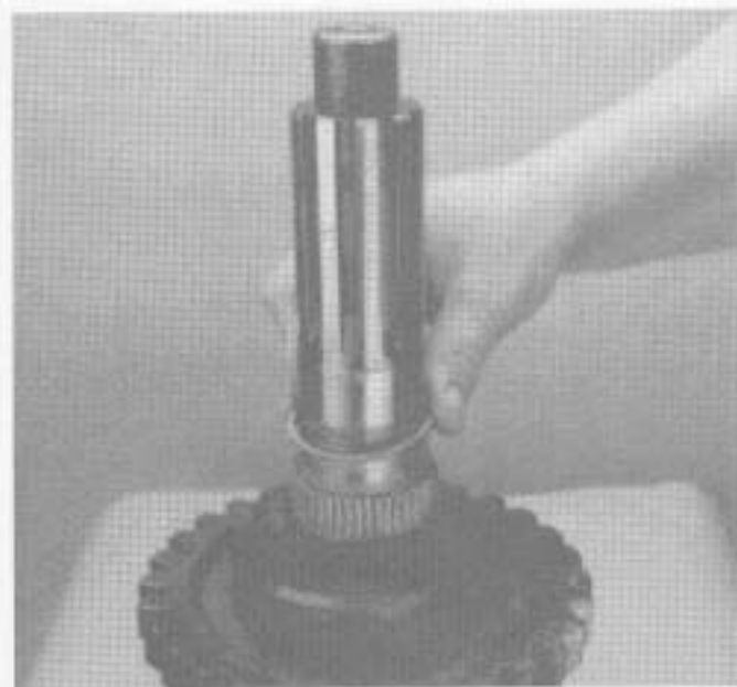
10. Coat the mainshaft 1st gear position with a high quality grease. Lay a row of needle bearings around the mainshaft, 44 needle bearings. Place a spacer ring over the top of the bearings. Lay a second row of 44 needle bearings around the mainshaft on top of the spacer ring. Install a spacer ring over the top of the second row of needle bearings.
