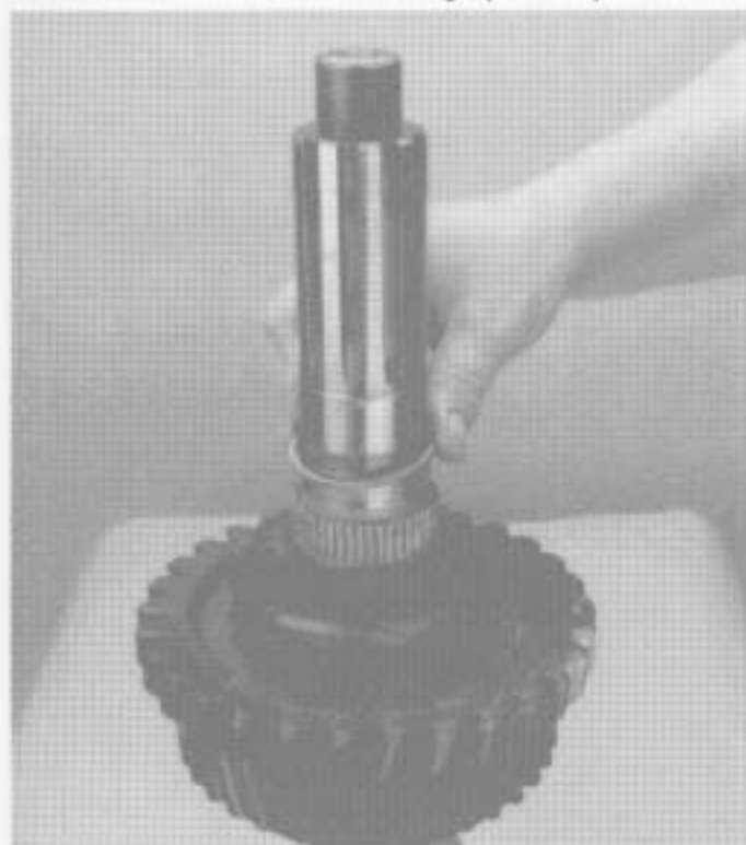
19. Remove the bearing rollers and spacers.
