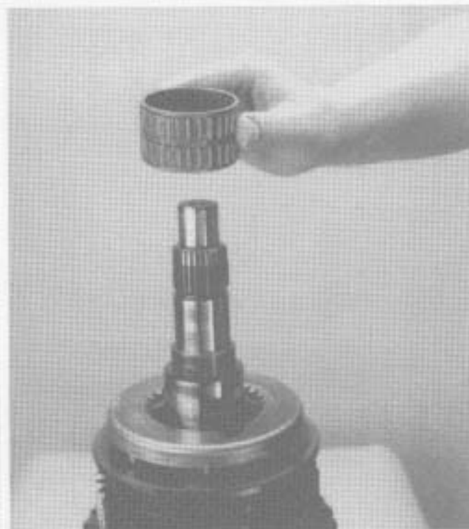
17. Install mainshaft 3rd speed gear bearing.
