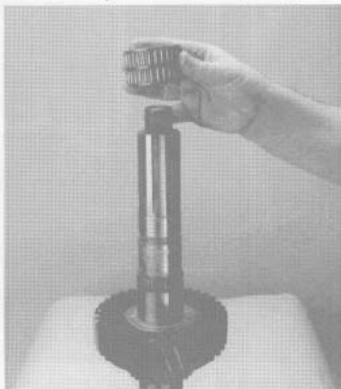
5. Install mainshaft reverse gear bearing.
