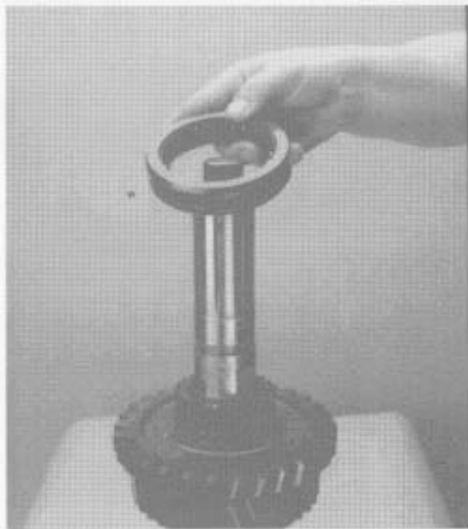
8. Install 1st-reverse gear sliding clutch.
