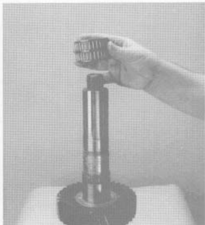
24. Remove the reverse gear bearing.
