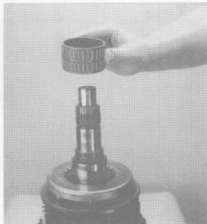
12. Remove the 3rd gear bearing.
