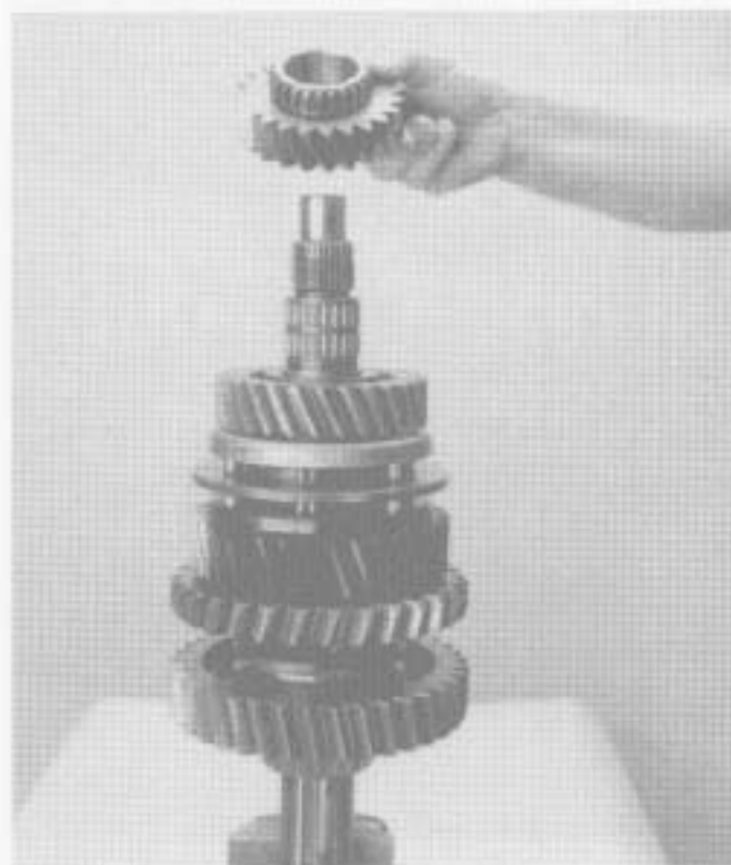
7. Remove the 4th speed gear.
