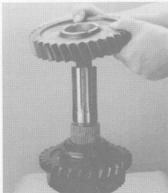
11. Install mainshaft 1st gear over the two rows of needle bearings, with clutching teeth down. Be careful not to catch the needle roller bearings.
