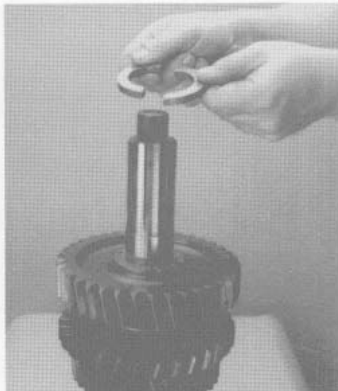
17. Remove the 1st gear split washer.
