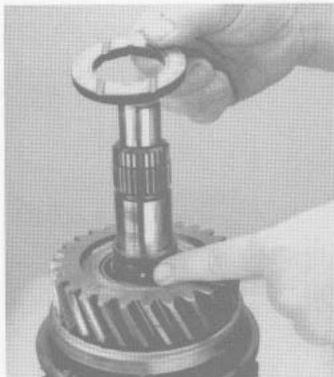
19. Install locating ball and 3rd speed gear thrust washer.
