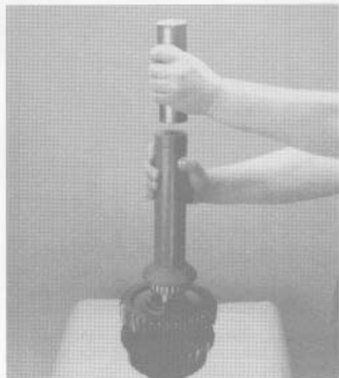
14. Using a bearing driver, install mainshaft rear bearing as shown.
